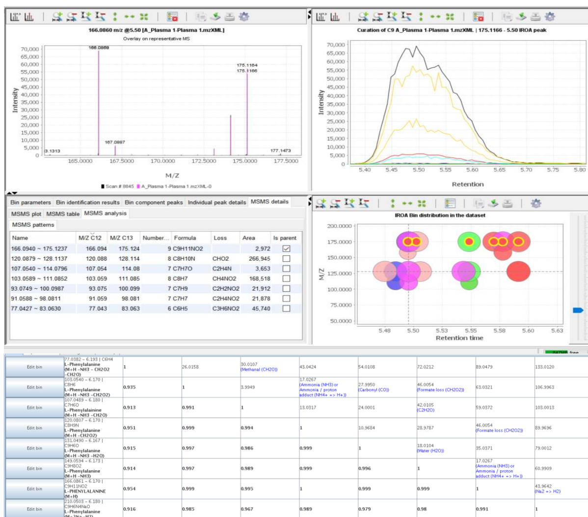
Figure 6: Data Review in ClusterFinder Software. The fragmentation of phenylalanine is seen in the central SWATH acquisition scan (A). ClusterFinder detected all of the IROA peaks in this scan (B & C). Note that for each peak the number of carbons in the fragment can be determined, and therefore the formula for the fragment is known (D). ClusterFinder Represents them both as (D) & (E). The actual fragmentation path (F) is easily determined from (E).
