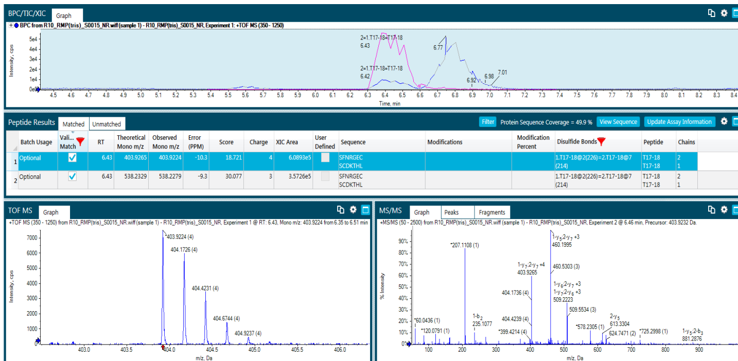
Figure 4. Automated identification of the disulfide bond C226-C214 between the heavy and light chain of the Fab. An extracted ion chromatogram (XIC) trace displays peaks obtained during TOF MS analysis of the tryptic digest (upper panel). BioPharmaView™ Software automatically identified two charge states for the C226-C214 disulfide-containing peptide with a good MS/MS score (middle panel, +3 and +4). A high-resolution TOF MS spectrum of the disulfide-containing peptide is displayed (lower left panel), and the corresponding MS/MS spectrum shows the fragment ions for that peptide (lower right panel).
