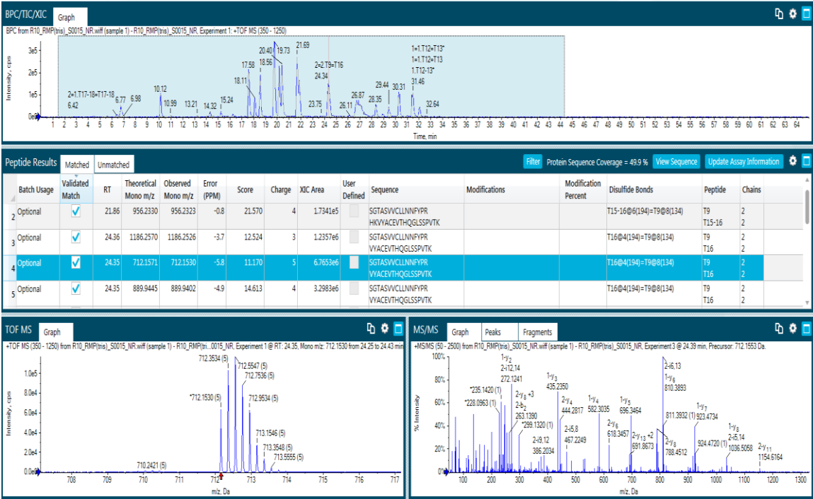
Figure 2. Automated identification of the disulfide bond C194-C134 in the light chain of the Fab. An extracted ion chromatogram (XIC) trace displays peaks obtained during TOF MS analysis of the tryptic digest (upper panel). BioPharmaView™ Software automatically identified four charge states for the C194-C134 disulfide-containing peptide with a good MS/MS score (middle panel, +3, +4, +5, and +6). A high-resolution TOF MS spectrum of the disulfide-containing peptide is displayed (lower left panel), and the corresponding MS/MS spectrum shows the fragment ions for that peptide (lower right panel).
